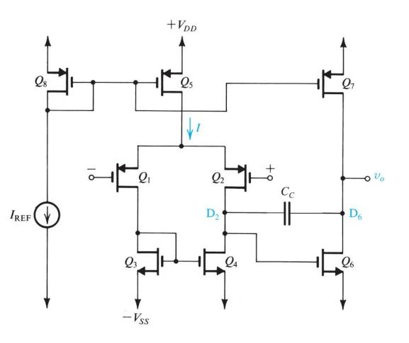
Voltage gain of the first stage  $(Q_1, Q_2)$ : Differential input, single-ended output:
